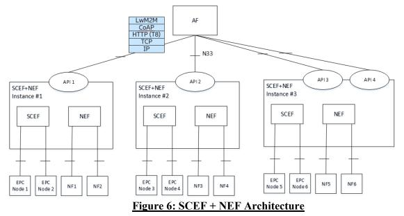
The API interface that is exposed by the SCEF+NEF interface is a N33/Nnef interface that supports the 3GPP T8 APIs (refer to TS 29.122). LwM2M over CoAP may be embedded in T8 APIs as the delivered data payload.
