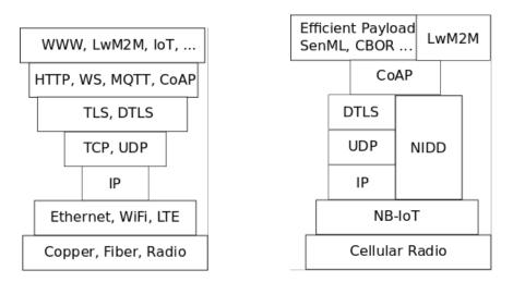
In this model, CoAP (Constrained Application Protocol) based protocols such as LwM2M become new spanning technology. With built-in congestion control, block-wise transfer fragmentation handling mechanism, efficient coding of headers and payload, and being effectively transport agnostic, CoAP-based LwM2M stack can be reused for both IP- and Non-IP- based NB-IoT deployments.
