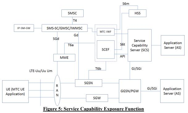
SCS is the entity which connects MTC application servers to the 3GPP network to enable the application servers to communicate through specific 3GPP-defined services with UEs that are used for MTC. SCS communicates with SCEF using standardized APIs.
