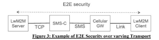
LwM2M 1.1 adds a core LwM2M OSCORE (ID:21) object. The LwM2M Security Object, OSCORE security mode is an optional resource that links to the LwM2M OSCORE object instance. Similar to the LwM2M Security Object, the LwM2M OSCORE Object must only be accessible and updatable by one LwM2M Bootstrap-Server.
