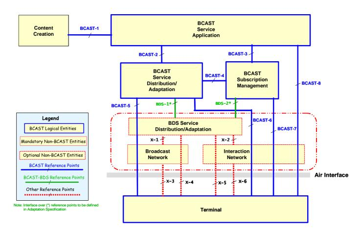
Figure 3: BCAST Functional Architecture Diagram
