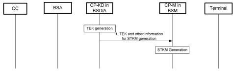
Figure 62 – Function Flow for STKM Generation by BSM
