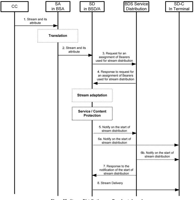
Figure 25 - Stream Distribution over Broadcast channel
