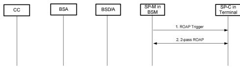
Figure 32 - Re-Keying Flow for DRM Profile with Interaction Channel
