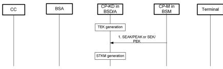
Figure 63 – Function Flow for STKM Generation by BSD/A
