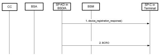
Figure 36 - Re-Keying Flow for Broadcast-only Terminal
