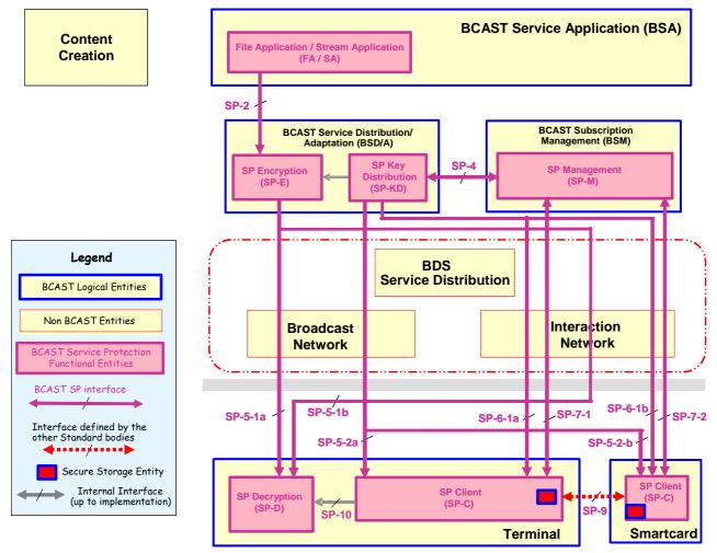
**Figure 8 - Service Protection Functional Architecture**
