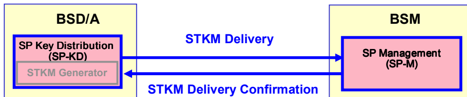
Figure 23 – Alternative Message Flow between BSM and BSD/A for Delivery STKMs
