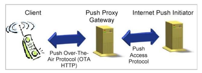
The model is analogous to the push model described in [SYNCWSP] with the difference being that instead of the push services between the Push Proxy Gateway (PPG) and the device being defined by the OTA-WSP protocol they are defined by the OTA-HTTP protocol. Full details of the specifics of both of these are described in [PUSH].
