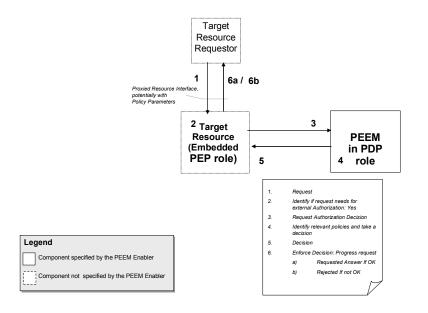
Figure 13. PEEM support for PEP/PDP behavior - Scenario B
