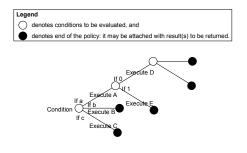
Figure 7. An Example of a graph that describes the topology of a policy (composed of multiple policy rules).
