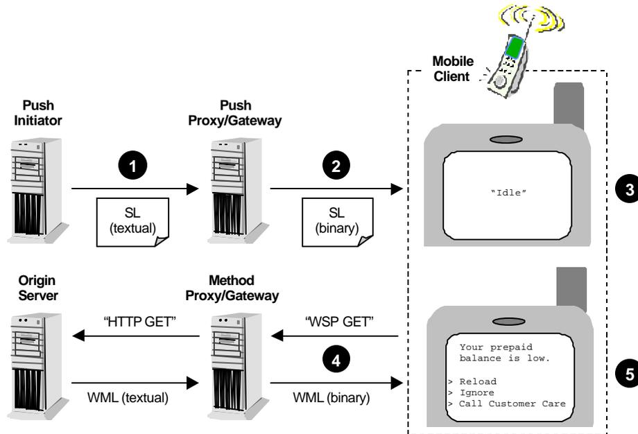
**Figure 1 : Service Loading - the basic concept**
