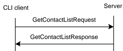
Figure 4. The “GetContactList” Transaction
