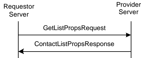
Figure 33. The “GetListProperties” Transaction
