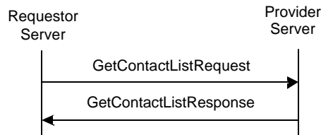
Figure 29. The “GetContactList” Transaction
