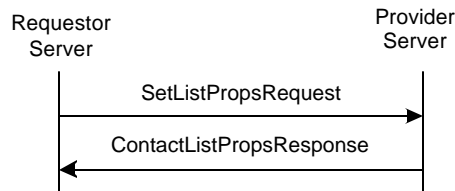
Figure 34. The “SetListProperties” Transaction
