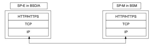
Figure 17 – Protocol Stack for SP-4-1
