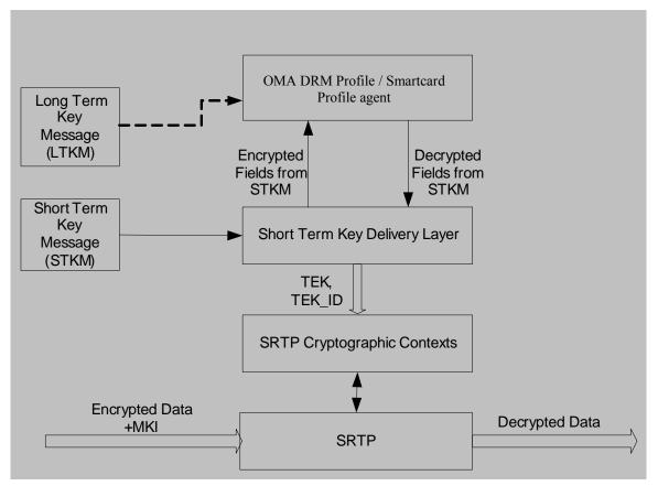
Figure 11 – SRTP Cryptographic Context Management (General Case)
