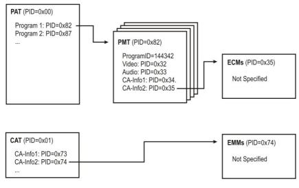
Figure 6: Example of the use Program Association Table (PAT), Program Map Table (PMT) and Conditional Access Table (CAT) to signal carriage of ECMs and EMMs
