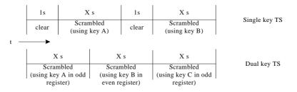
Figure 7 - Single key vs. dual key TS over time
