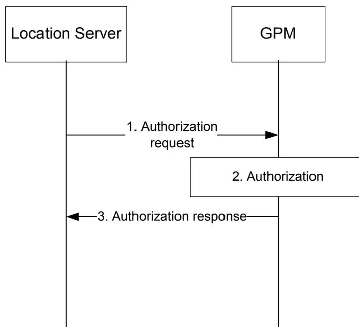
**Figure 11: Flow for permissions checking with GPM**
