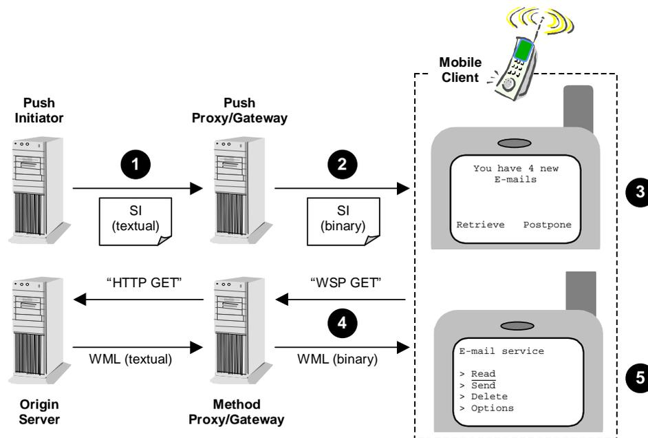
**Figure 1 : Service Indication - the basic concept**
