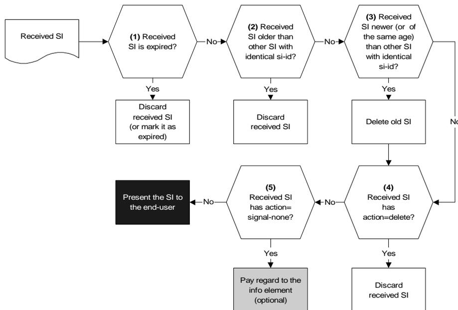
Figure 2 : Steps involved in processing a received SI
