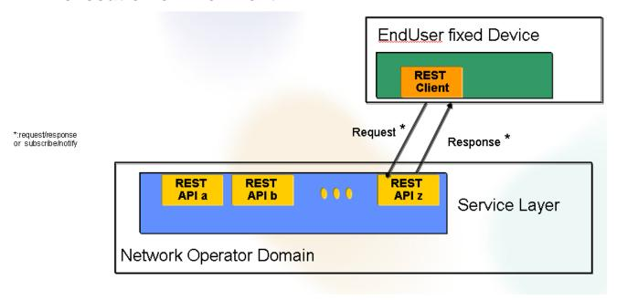
Figure 3 RESTful Network API accessed from a fixed device execution environment
