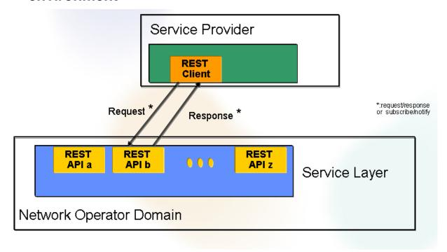
Figure 1 RESTful Network API accessed from a server execution environment (e.g. 3<sup>rd</sup> party Service Provider application)
