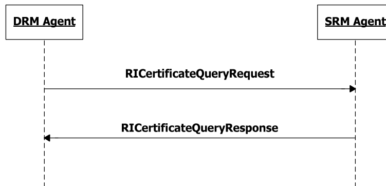
Figure 38: Sequence Diagram – Get RI Certificate Chain
