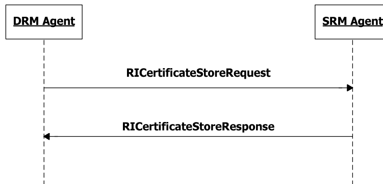
Figure 37: Sequence Diagram – Store RI Certificate Chain
