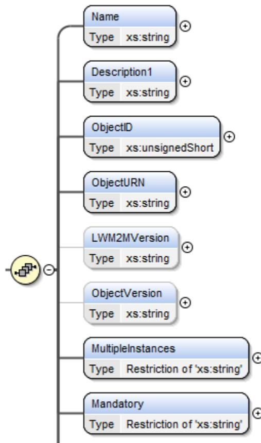
Figure 3: Elements in the Object Definition Part
