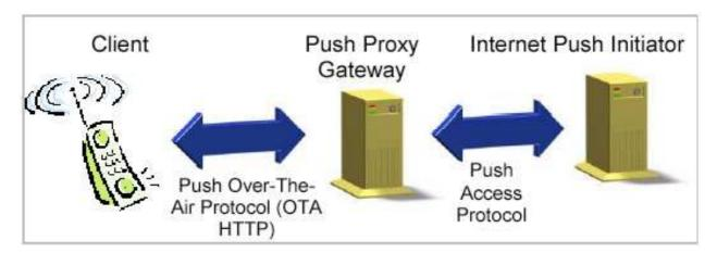
The model is analogous to the push model described in [WSPBIND] with the difference being that instead of the push services between the Push Proxy Gateway (PPG) and the device being defined by the OTA-WSP protocol they are defined by the OTA-HTTP protocol. Full details of the specifics of both of these are described in [PushOTA].
