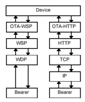
Note that the push model is not limited to OTA usage, the model could also be used locally with, for example, a DM Server running on a PC connected to a DM Client via a cable. In this situation the DM Server would be REQUIRED to emulate the PPG services. This mechanism might prove useful to vendors who require a means of achieving local Server Alerted Notification over TCP.
