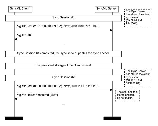
Figure 3 Example of Sync Anchor Usage
