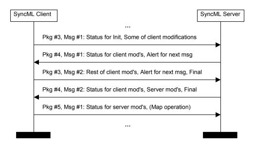
Figure 5 Example of Sending Multiple Messages in a Package
