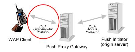
Figure 1: System architecture
