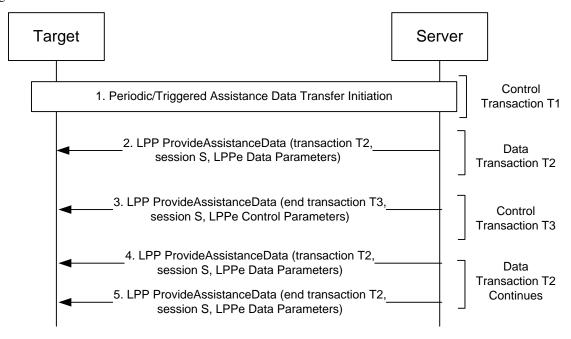
Figure 3: LPPe Periodic/Triggered Assistance Data transfer procedure with Server Update
