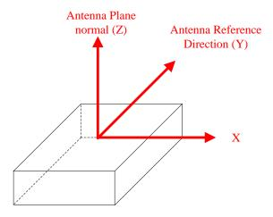
Figure 15: Antenna reference frame
