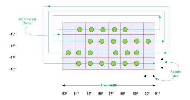
Figure 11: Run length encoding
