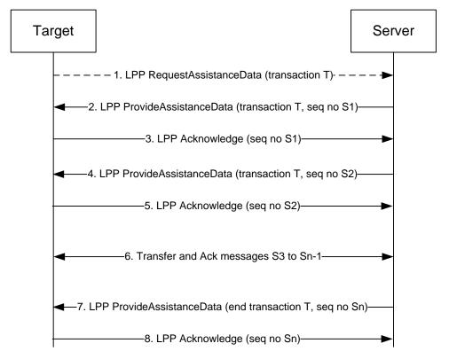
Figure 7: LPPe Segmented Assist ance Data Transfer
