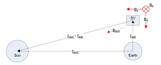
Figure 14: Satellite-fixed coordinate system
