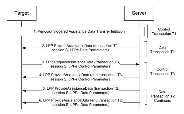
Figure 2: LPPe Periodic/Triggered Assistance Data transfer procedure with Target Update
