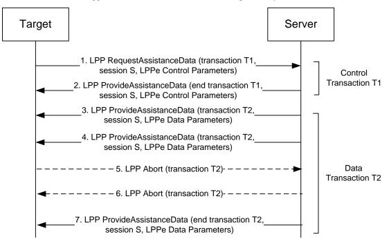
Figure 1: LPPe Periodic/Triggered Assistance Data transfer procedure with Update
