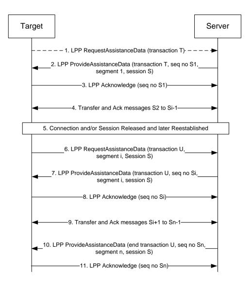
Figure 8: LPPe Segmented Assistance Data Transfer with Resume Capability
