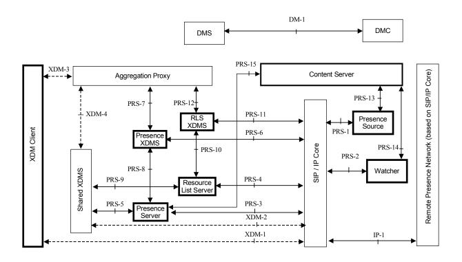
Figure 1-SIMPLE Presence Reference Architecture
