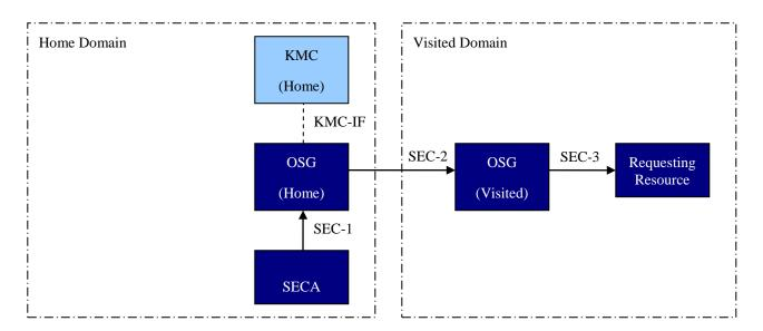
Figure 4: GBA deployment for SEC\_CF roaming domain architecture
