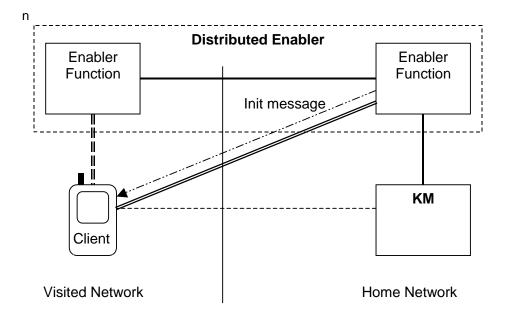
Figure 5: Network initiated connection between MT and Enabler.
